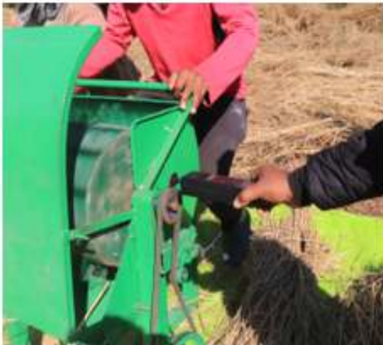
a. Measurement of cylinder speed by tachometer
